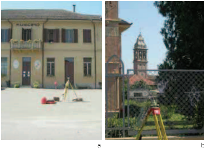
Figure 7 Extremes of the GPS baseline for the determination of the coordinates of the cadastral origin, using a forward intersection.
